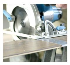
Next, you'll **cut the planks using a table saw, miter saw, circular saw or handsaw.** Moulding will cover the edges so every cut doesn't have to be perfect.
