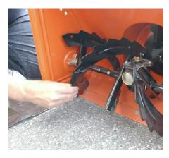
**Lubricating moving parts regularly** will make sure all parts turn and move correctly. Wheel bearings, auger bearings, and the impeller bearings should all be greased. Inspect the belts and scraper bar for wear and then replace any worn out parts.
