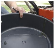
**Begin by completely draining your old oil and gas,** then dispose of them before adding fresh fluids. Most small engine and auto parts stores offer a free recycling program. If you have a 4-stroke machine check your oil level after every 8 hours of use. If your machine has an air filter, replace it as well.
