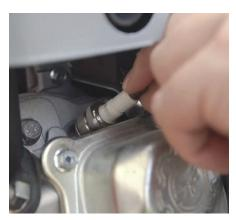
A worn out spark plug causes increased emissions, reduces engine performance and increases fuel consumption. So you should **replace your plug** at least once per year and check the gap periodically. Consult your owner's manual to ensure that you're using the correct plug for your machine. Use a spark plug wrench for safe and easy plug removal and installation.
